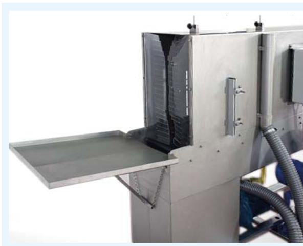
Exit table for water draining.
