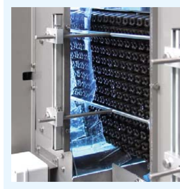
Trays treatment tunnel with UV lamp system.
