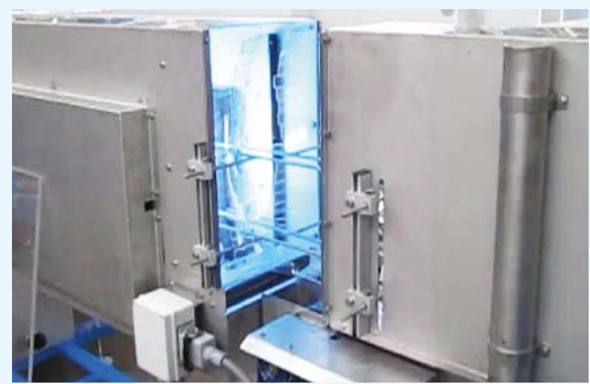
Trays treatment tunnel with UV lamp system.
