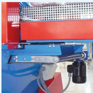
16 Belt for the recycling soil for trayfiller.
