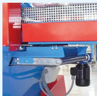
16 Belt for the recycling soil for trayfiller.
