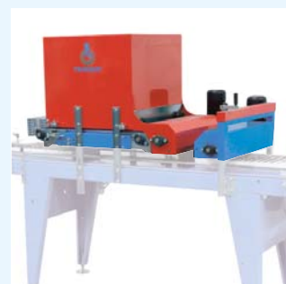
18 Sand and soil coverer with brush to clean the trays.
