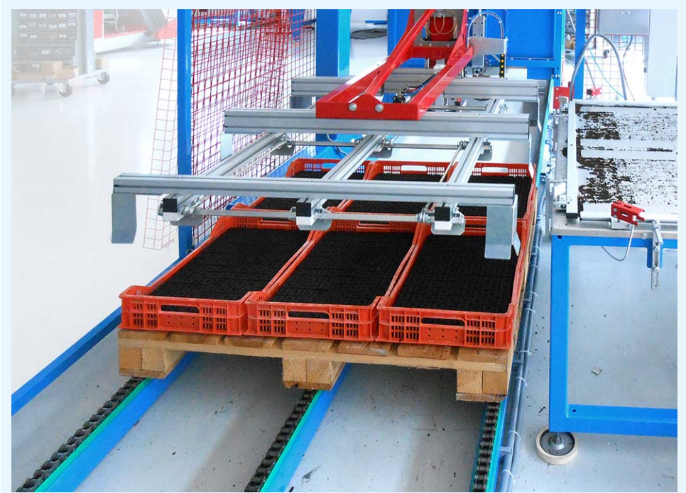
Palletizer for crates with blocks : collet on unloading phase .
