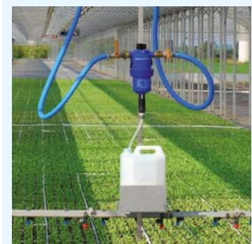
Proportional dosing unit assembled directly on the irrigation boom .
