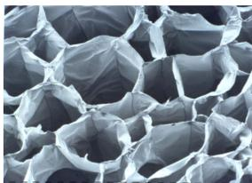
Photomicrograph of internal Structure of Broadleaf P4 water-storing polymer showing honeycomb water-holding formation
