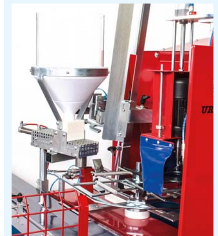
46 Fertilizer batching plant accessorized with tank 15 l.
