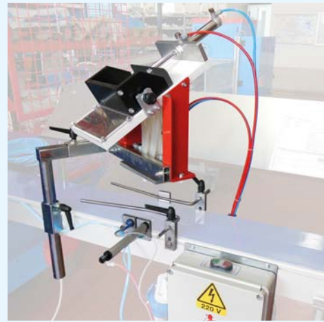
41 Mechanical seeder for aromatic plants, complete with electric panel, pot block and descent seed guided with tubes or spread.
