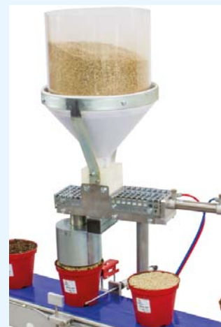
45 Drum coverer for vermiculite.
