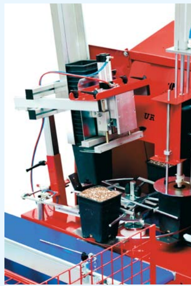
Special denester for pots not easy to separate.
