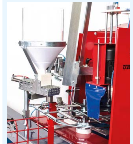
46 Fertilizer batching plant accessorized with tank 15 l.
