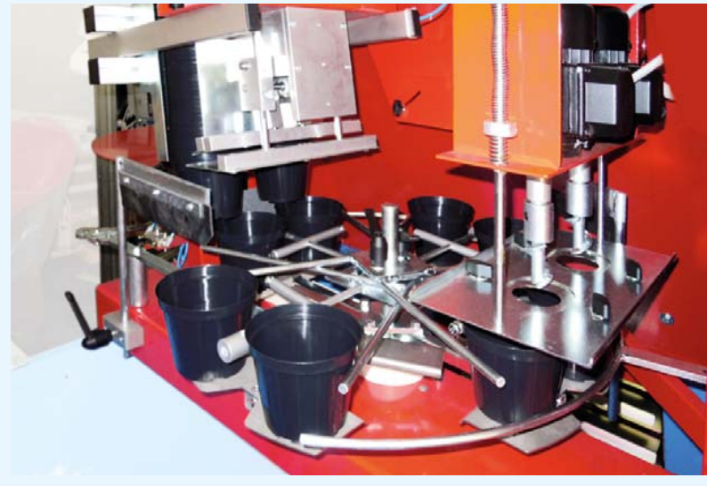
Double head version for pot from diam. 8 to 14 cm: up to 3500 pots/hour.
