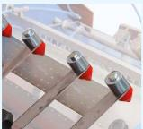
Adjustable speed hammers. The vibration helps placing the seeds in the center of the holes.
