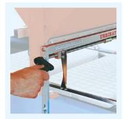
Fast and self-centering (29) system for width adjustment of the trays with handles.
