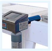
Black ink jet printer mod. (25) U2011: fixed version for moving trays to write on the long side of the tray.
