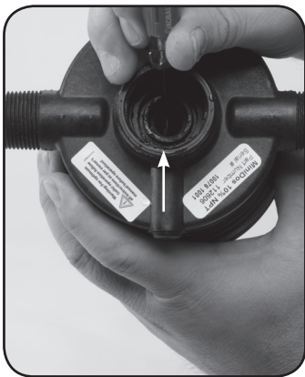
Step 4. Remove #17 O-ring and replace.
