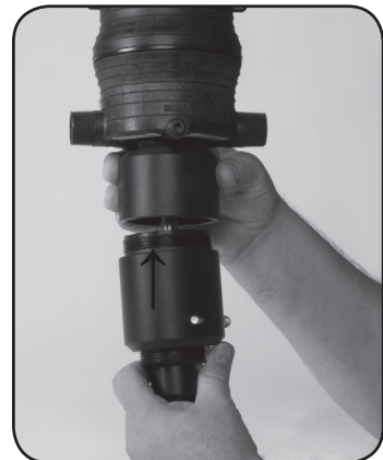
Step 9. Screw #61 OUTER CYLINDER onto body.
