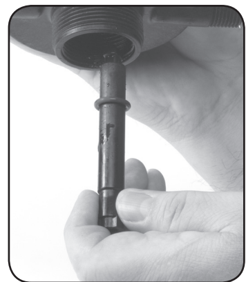
Step 6. Re-install #52 UPPER SHAFT and #17 O-ring.
