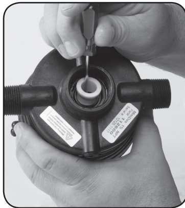
Step 4. Remove #82 SHAFT SEAL SPACER.
