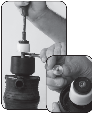
Step 2. Unscrew to unlock and remove #93 CAPSCREW.
