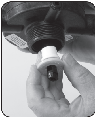
Step 7. Re-install #82 SEAL SPACER and #16 GASKET.
