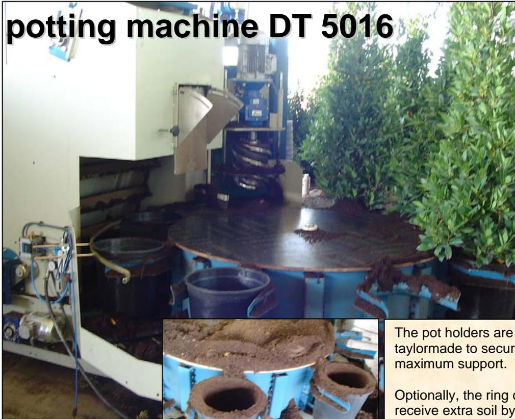
The up and down going movement of the drill is frequency controlled. The powerful motor enables drilling holes with maximum diam. 32 cm. The machine can be set in such a way that for instance a plant out of a 32 cm pot can be potted into a 40 cm pot. The pot dispenser is obviously adjusted for such containers. The number of pots on the potting ring is determined by the space that the plants require, multiple combinations are possible.
