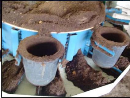
The pot holders are tailor-made to secure maximum support.
