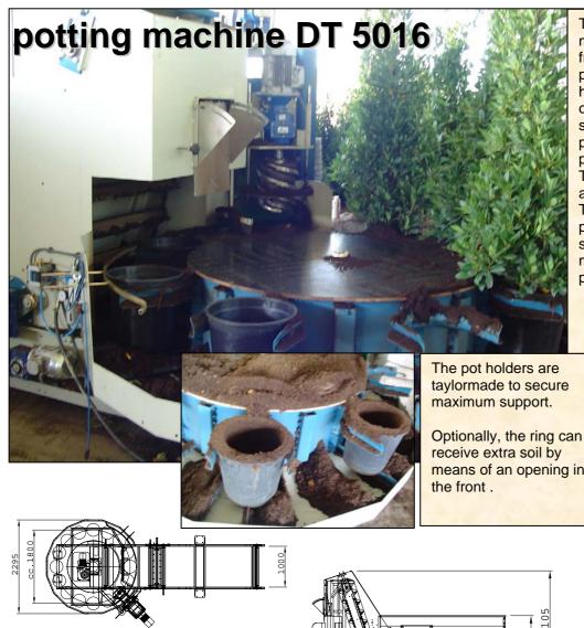
The up and down going movement of the drill is frequency controlled. The powerful motor enables drilling holes with maximum diam. 32 cm. The machine can be set in such a way that for instance a plant out of a 32 cm pot can be pot into a 40 cm pot. The pot dispenser is obviously adjusted for such containers. The number of pots on the potting ring is determined by the space that the plants require, multiple combinations are possible.
