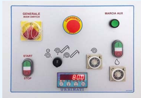
Control panel equipped with display for the electronic weighing .
