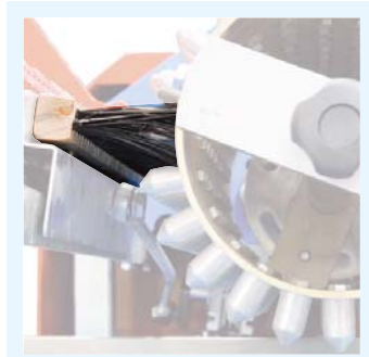
7 Oscillating cleaning brush for the dibbler, useful with wet soil.
