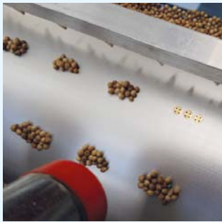
11 Sowing drum with multi-hole nozzles for aromatics, microgreens etc.
