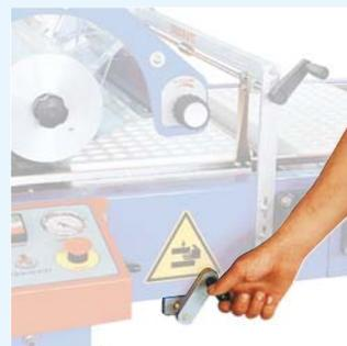
Easy and fast adjustment of seeding system's height and dibbler's depth, thanks to **comfortable handles**.
