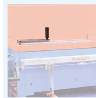
The adjustment of the tray's height, width and soil density is made with **functional handles**.
