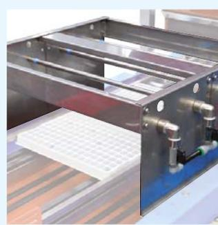
The drilled bar system, produced by CNC machines, makes the **watering uniform**.
