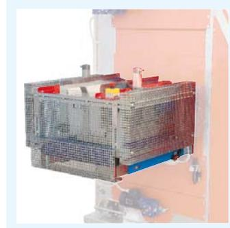
**Electropneumatic denester with 3 movements** for thermoformed trays (PE - PET).
