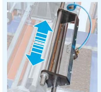
**Oscillating seed holding plate** to distribute the seeds **uniformly** all over the working width. It enables to work also with a small quantity of seed.
