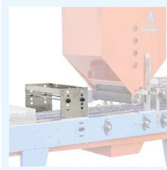
**Second water unit** with nr. 2 drilled bars: mainly needed to increase the soil watering. **23**
