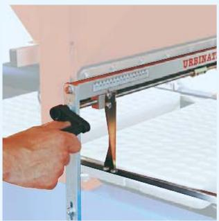
**Fast and self-centering system** for width adjustment of the trays with handles.
