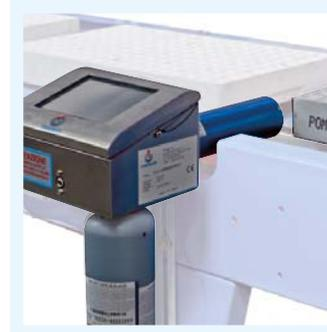
**Black ink jet printer mod. U2011:** fixed version for moving trays to write on the long side of the tray. **25**
