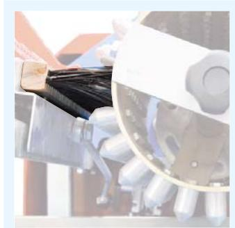
**Oscillating cleaning brush** for the dibbler, useful with wet soil.
