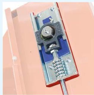
**Engineering solutions** aimed to reduce and simplify the maintenance. For example, visible bearings lubricator, spring tensioner on chains, etc.
