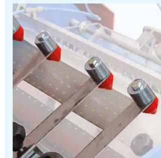
**Adjustable speed hammers.** The vibration helps placing the seeds in the center of the holes.
