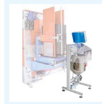
**ETC automatic labelling machine:** to print and apply labels on the trays coming out from the denester. **24**
