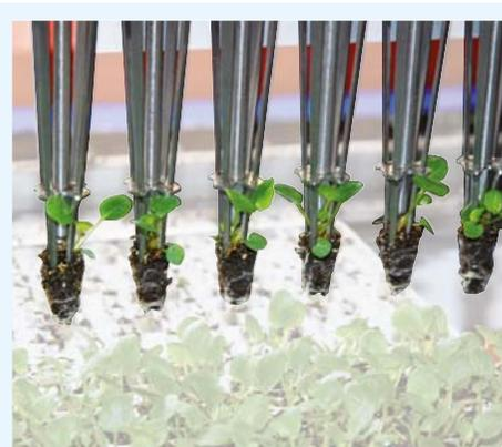
**The exclusive flat profile** of the needles and the closing system **allow an excellent grip** of the plug even with weak-rooted plants.
