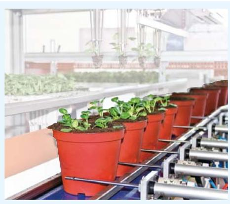
**Pot positioning** on the belt with cylinders (diameter pots from 9 to 20 cm).
