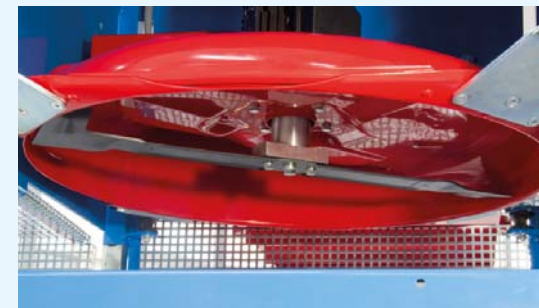
Trimmer with rotating blade.
