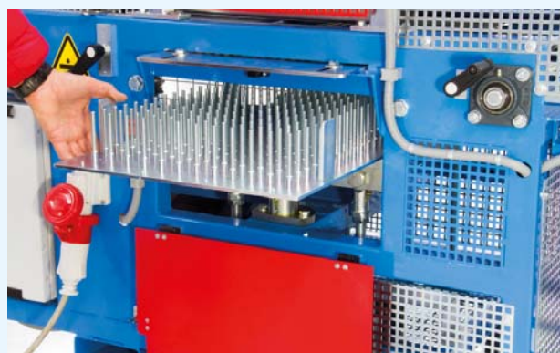
Rapid side replacement of plates.
