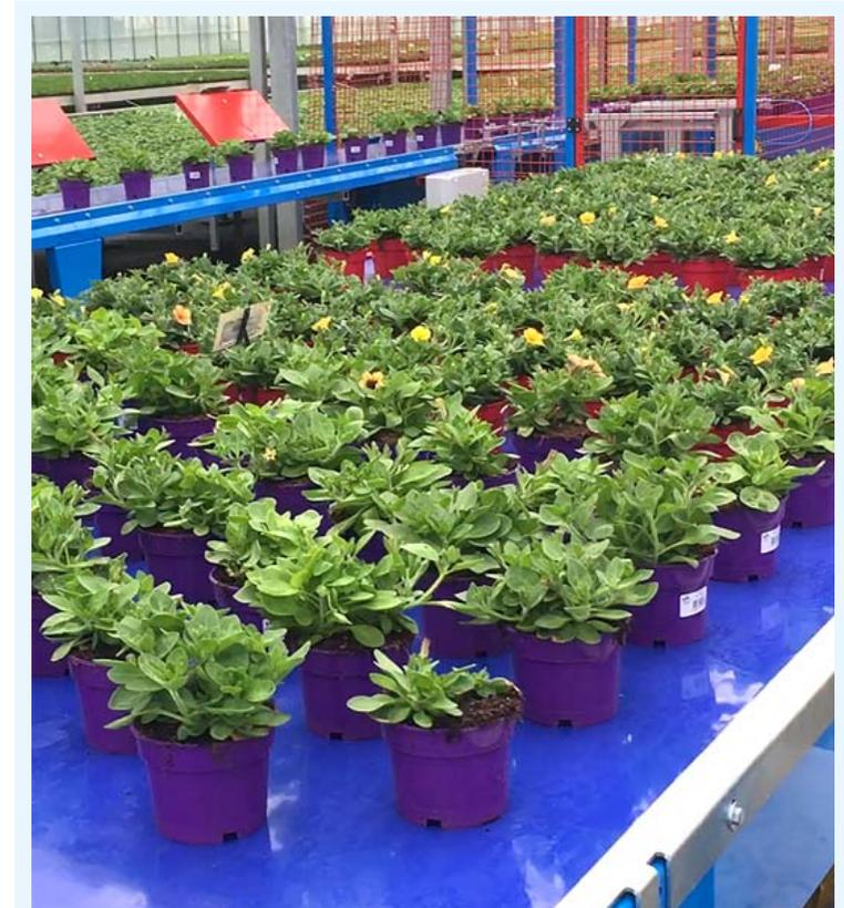
Example of plant processing line in pots, consisting of a buffer belt with take off and a successive buffer belt with push over.
