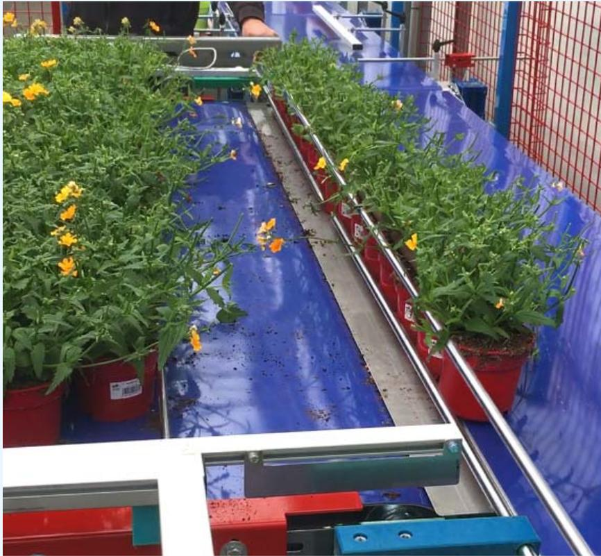
BUFFER BELT with take off and THREE-BARS DEVICE:
