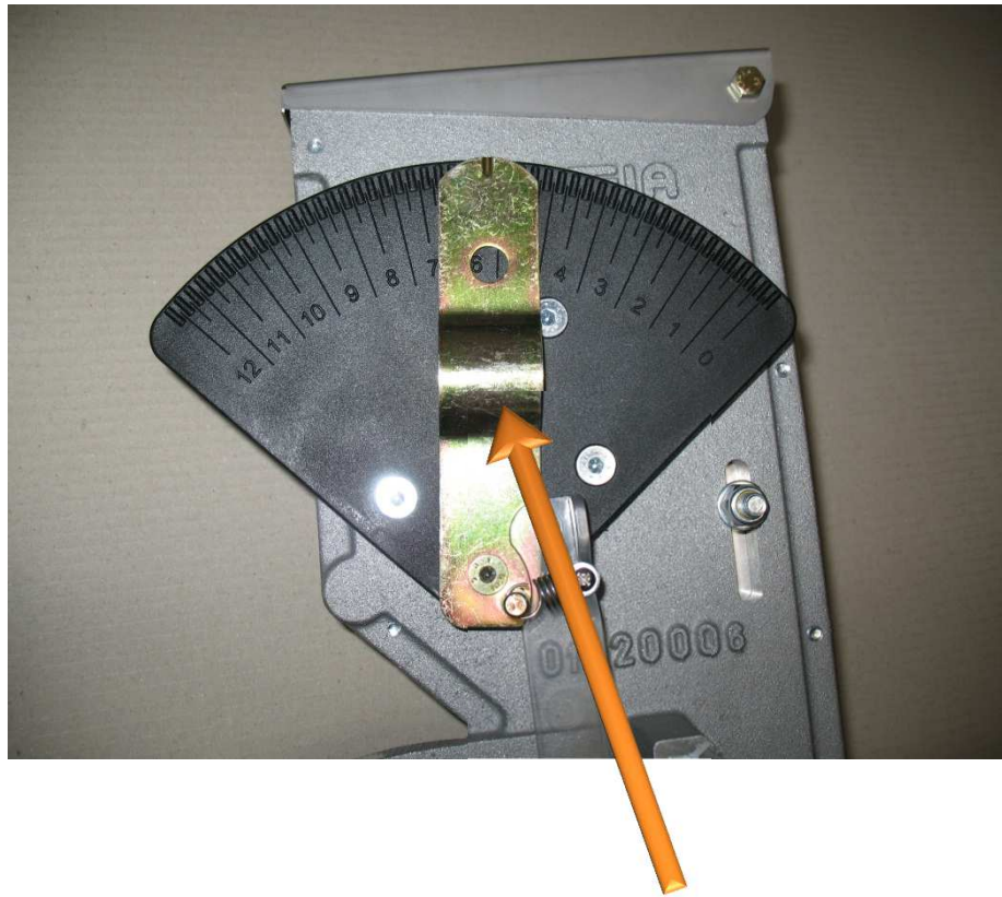
Teeth selector regulation lever
