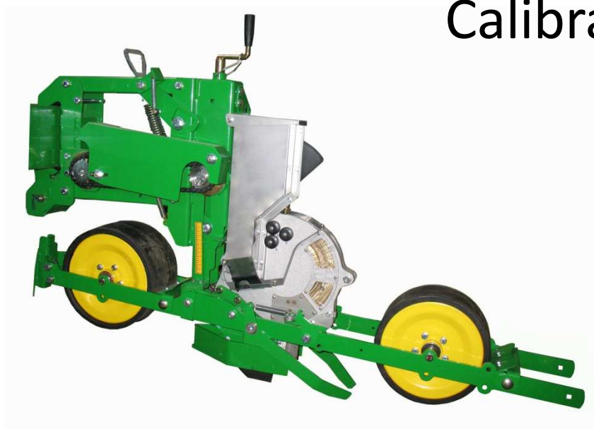
Twin line shoe for sandy soils
