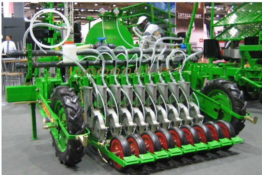
5 cm Twin line shoe for sandy soils
