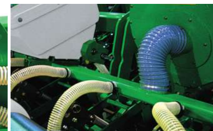
Really silent vacuum fan with an elevate power, can feed up to 18 rows, with a 540 RPM P.T.O. shaft (750 RPM or 1000 RPM if requested). On the fixed frame version from 12-row corn up to 18-row for sugar beet and for all telescopic versions Sfoggia uses a metallic collector.
