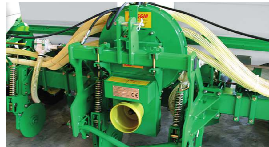
2nd and 3rd category 3 point hitch with quick connection device. 3rd category point hitch for big machines.
