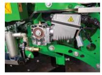
Electric motor + watering device
