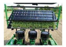
High-capacity plant tray carrier with racks for flexible trays
