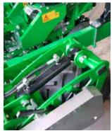
Hydraulic depth adjustment on "tractor" wheels
