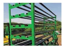
High-capacity plant tray carrier with tubulars for rigid trays
