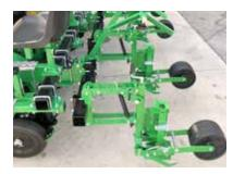
Mobile hose burying device on parallelogram.
