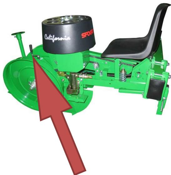
The planting depth is adjustable with an handle that lift or low back compression wheels.
