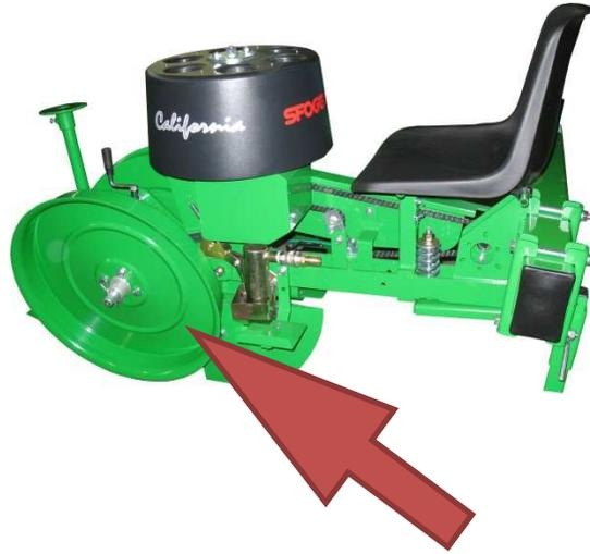
The plate of falling pipe has the function to help plants to stay straight when they fall in to the shoe.
