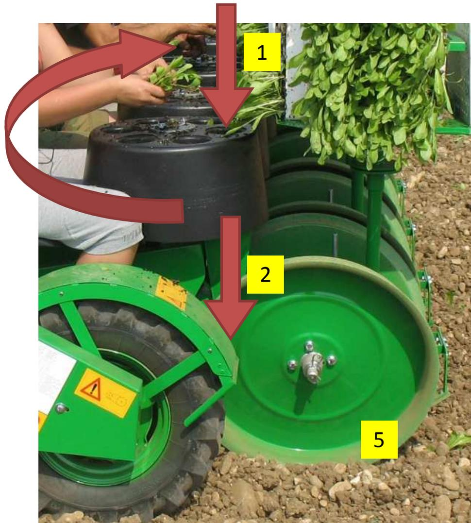
When cups of rotating carousel run over falling pipe [1] they open and plants get down through falling pipe [2] in the shoe [3].
