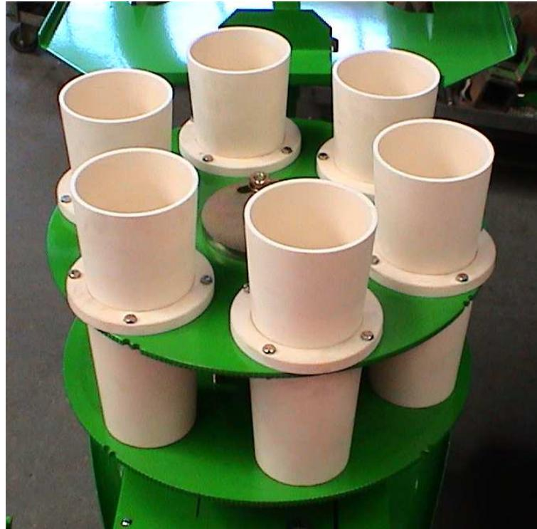
Carousel of plant distribution with 6 cups on crawling steel plate (option)
