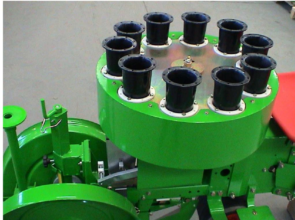
Carousel of plant distribution with 6 or 10 cups on crawling steel plate (option)
