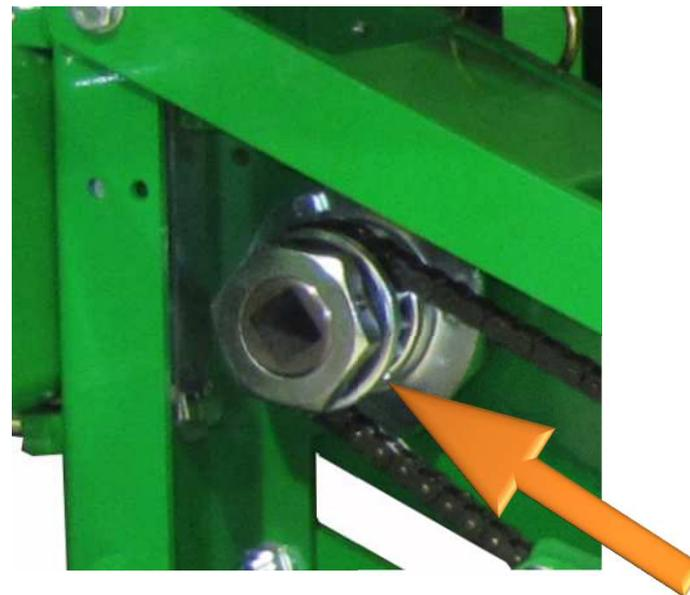
Planting unit has a security clutch: in case of objects/stones/etc that block the carousel rotation, it intervenes and doesn't allow breakage.
