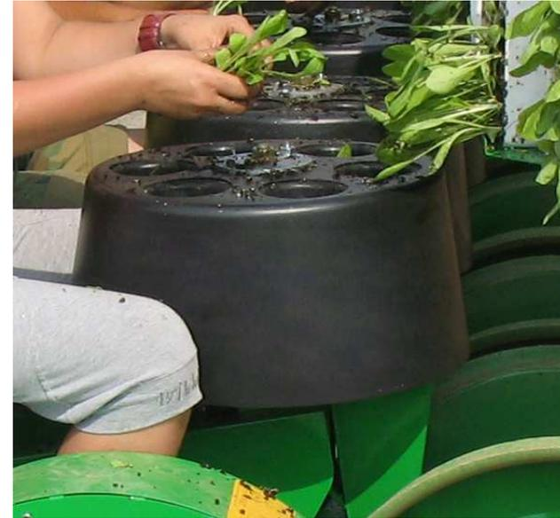
The carousel is made by teflon-nylon material:
